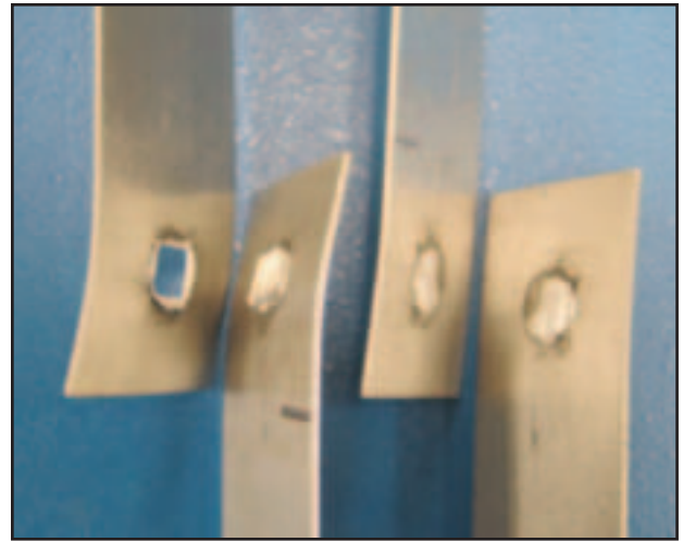
Fig. 21 — Button pull-out (left) and interfacial fracture (right) failure modes.
